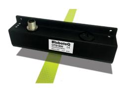
For use in less hostile environment, Roboteq offers a sensor capable of detecting the position of a reflective tape. Tape is available from Roboteq in yellow, blue, green and red colors. The different colors can be used on the same track to create different paths, or as location markers. The sensor operates at distances from 30 to 100mm
